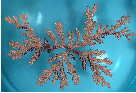
(a) Electrodeposition of copper ions (Experiment)
